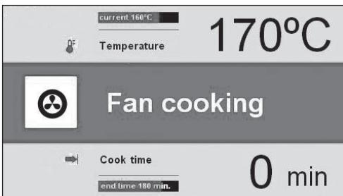
Touch **ok** sensor field to adjust temperature again. Touch **ok** to start the program. The following operate: cooling fan motor, lighting, fan cooking motor and fan heater. Fan heater is operates intermittently (thermostat) ensuring stable temperature in the oven chamber. Current oven chamber temperature is displayed, „current 160 °C”.
